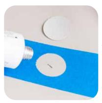
Apply glue to the patch and boat. Allow to dry 15 minutes. Glue must be dry to the touch. If glue layer is thin, apply second coat, allow to dry 15 minutes.
