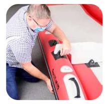
Look through the grommet hole to check alignment with hole in transom. Pull or push bottom of side chamber until holes line up.
