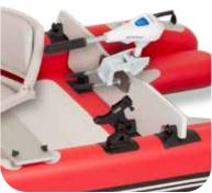
Clamp electric motor or up to a 6hp gas motor to motor mount. Turn clamp screws until tight.
