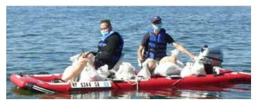
The FastCat12 has four floatation chambers; two side chambers and two floor chambers. The boat will stay afloat and can be paddled or motored when loaded to capacity with the main chamber deflated.
