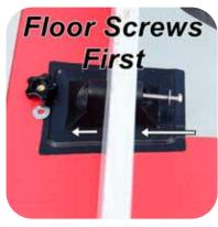
Start with floor grommets. Adjust transom board to align the holes.
