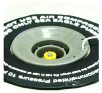
To deflate, push down on the valve stem and quarter turn it to the right. The stem will stay in the down position, allowing the air to escape.
