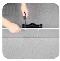
Place one washer and one nut on each screw. Tighten screw with #2 philips head screwdriver and a 7/16" or adjustable wrench. Screw must engage the nylon insert in the locking nut.
