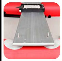
Lay one end of bench over the screws, so screws come up through the holes in bench.
