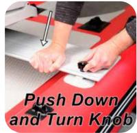
Push bench down against boat with one hand and tighten each knob.
